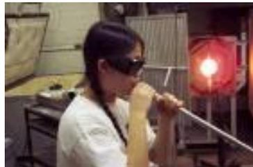
**Step 4** To keep the glass warm so it can be shaped, the gaffer moves the piece in and out of a **gloryhole**, or reheating furnace. If it cools too quickly, it becomes brittle and it could break. The gaffer can also reheat individual sections with a blow torch.
