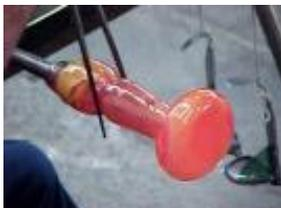
**Step 6** When the piece is finished, it is cut from the blowpipe and placed in an **annealing oven**. This special oven heats to high temperatures and then gradually cools the glass which helps keep it from breaking.
