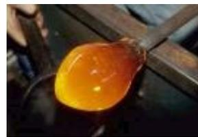
**Step 3** The gaffer twists the blowpipe while blowing into it. The gaffer's breath expands the molten glass into a **bubble**.
